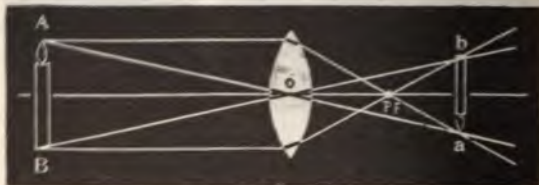
FIG. 157.—Real, Inverted and Reduced Image Formed by a Convex Lens.
